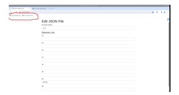
4. Fill the device list fields with the SN number from the watch display according to the slots where the watches are located. For example, if the watch is located in slot 4B and the watch has SN number '6A213C' on the screen, then we put '6A213C' in the 4B field. Repeat this process for all watches in their designated slots. Finally, press the 'SAVE' button.
